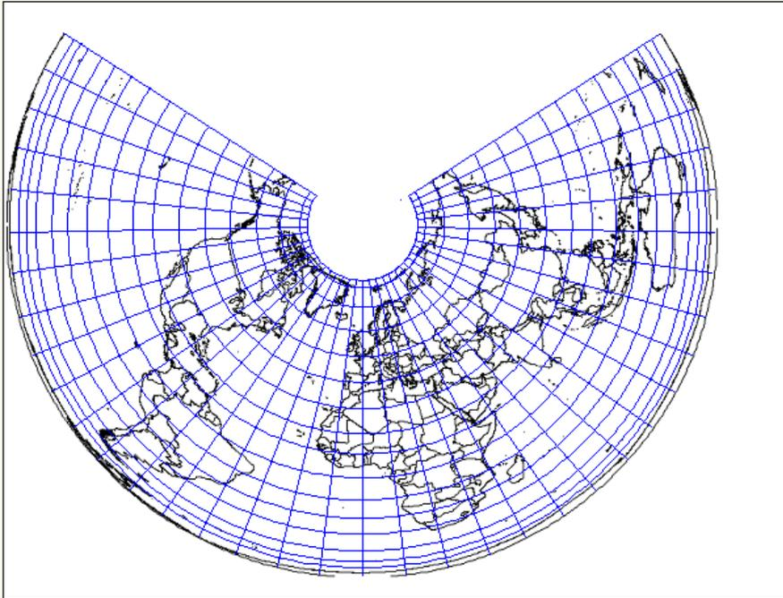
Fig 38. Albers Equal Area Conic with  $30^\circ\text{N}$  and  $60^\circ\text{N}$  Standard Parallels and  $0^\circ$  CM
