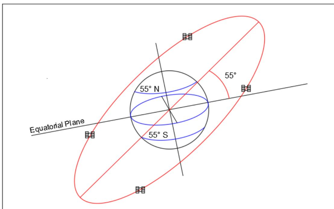
Fig 1. Inclination of Orbital Plane to Equatorial Plane.
